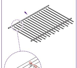
Insert the pickets into the Top Rail (D) and align the holes in the pickets with the holes in the top rail.
