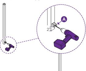
Attach the rail bracket with a ¾" self-drilling stainless steel hex screw. If you force the screws, you will strip them.
