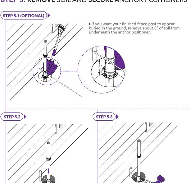
▶ Adjust your string line to the string line marking on the anchor positioner.
